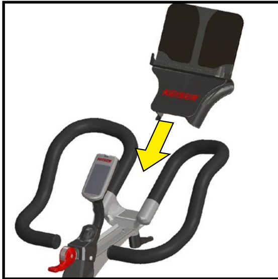
Figure 19. Assemble the device holder to the handlebar
