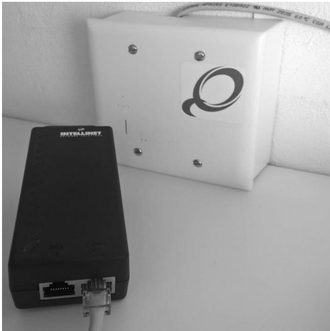
The Team Receiver must be connected via a PoE-Adapter (Power over Ethernet) on the same Ethernet-based Local Area Network as the computer running iQniter Cardio Training software is connected (i.e. connected to the same Router). A Power over Ethernet connector provides power and Ethernet connectivity using one standard network cable.
