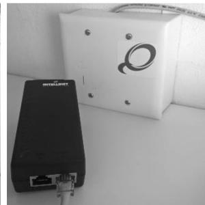
7. Connect the Ethernet cable to a PoE adapter (P+DATA OUT) (included) or to a PoE router (Self supplied).
