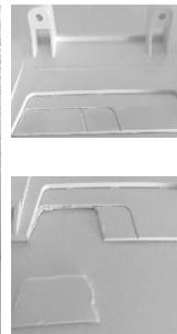
3. Cut or clip and break out a piece of the housing as shown, to make room for the Ethernet cable.
