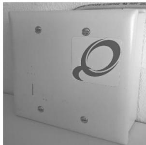
6. Click the receiver and the housing onto the mounted back plate. Be careful not to drag the cable too hard.
